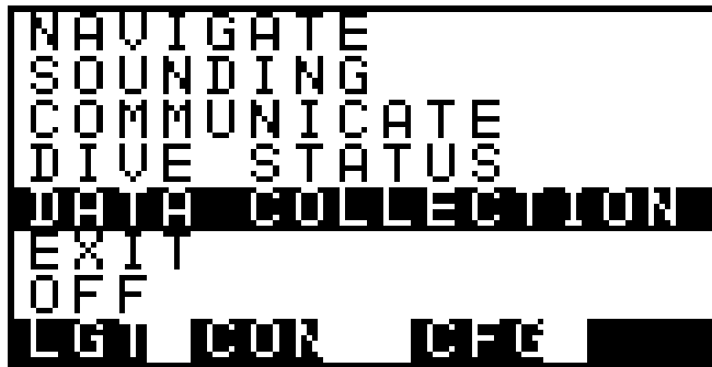
Figure 15: A Sample MODE Screen Of A DiveCode Application
