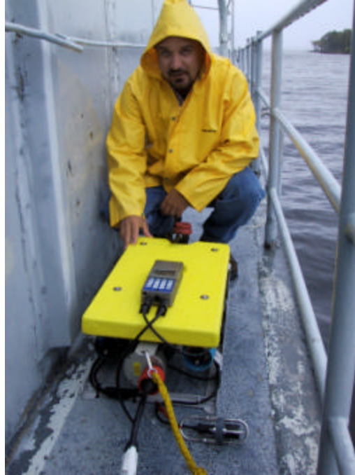
Figure 5: DS-1 Station mounted on an Outland ROV
