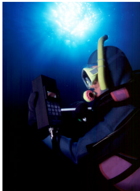
Figure 2: Diver Station Operated by a SCUBA Diver
