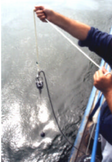
Figure 5: A Sonar Transducer is lowered over the side of the Surface Vessel
