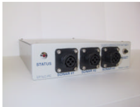
Figure 1: The STM-1 Surface Tracking Module For Permanent Installations
