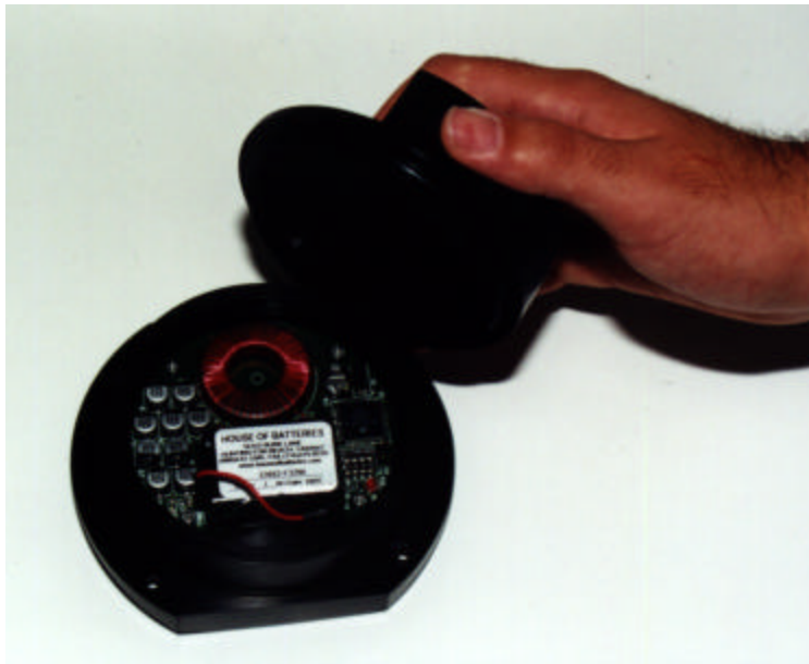
Figure 1C: The TLT-50 Transponder For MK50 Torpedoes
